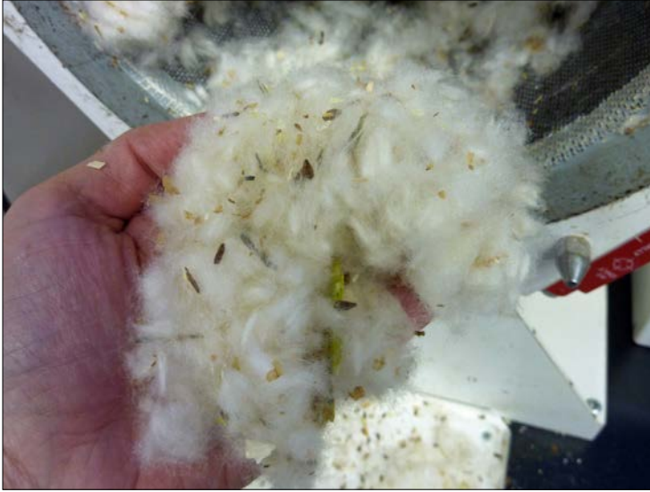
After brush machine processing, this coarse mixture of pod shells, floss, seeds, and small debris, is ready to be processed using an air-screen cleaner. (Photo: Brianna Borders, The Xerces Society.)
